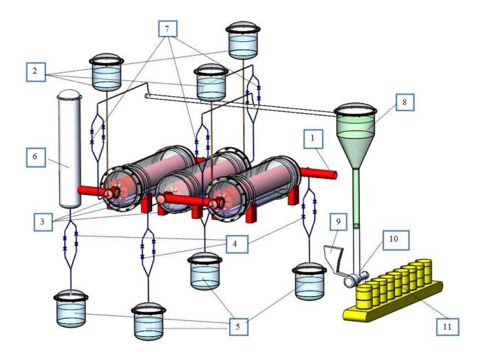
Figure 3. Scheme of a three-step DFE with secondary evaporation and steam heating: 1 - supply of heating steam; 2 – input solution tank; 3 –drum film evaporators; 4 – valves of condensate discharge; 5 – condensate collection container; 6 – condenser after the last step; 7 – valves of condensate supply; 8 – concentrate collection tank; 9 – cement mixture supply unit; 10 – cement compound preparing unit; 11 –containers filling by cement compound
