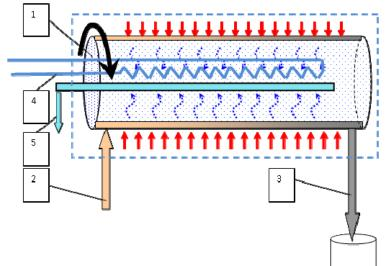
Figure 1. Diagram of the evaporation treatment of the liquid radioactive waste in the DFE: 1 - drum evaporator; 2 - supply of initial solution; 3 - discharge of the concentrate; 4 - secondary steam condensation circuit; 5 – secondary steam condensate discharge
