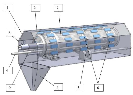
Figure 2. Scheme of the main components of drum-film evaporator: 1 - case; 2 - drum evaporator; 3 - drain channel; 4 - initial solution supply pipe; 5 - rotation drive of the drum; 6 - ceramic heaters (electric heating elements); 7 - tubes for condensed steam; 8 - central support tube; 9 - drive shaft for mechanisms of surface cleaning from sediments
