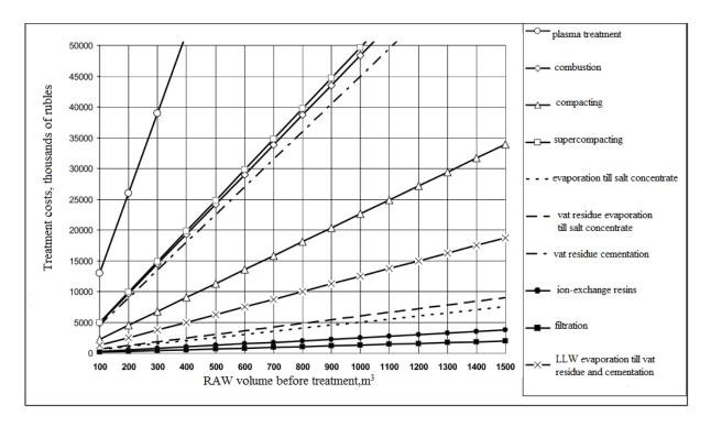
Figure 5. The cost of RAW preparing for final disposal, depending on applied technical solutions
