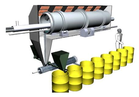
*Figure 6.* Continuous technological process of vat residue secondary evaporation in electrical heated DFE and concentrate conversion into cement compound
